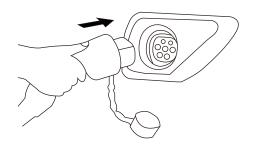
Step 3: Connect the charging adapter Type 2 plug to your EV to start charging. Check from the adapters screen that all is OK.
