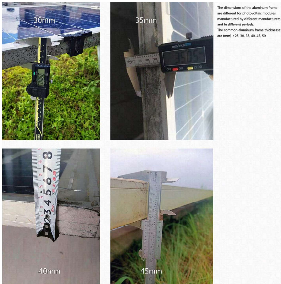
Figure 21 Measuring the thickness of the aluminum frame:
