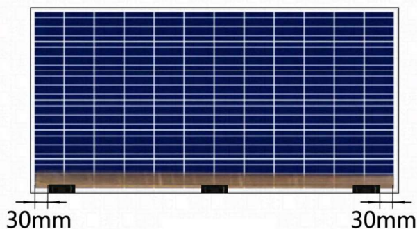
Figure 24 Larger than one meter may require the installation of three pieces
