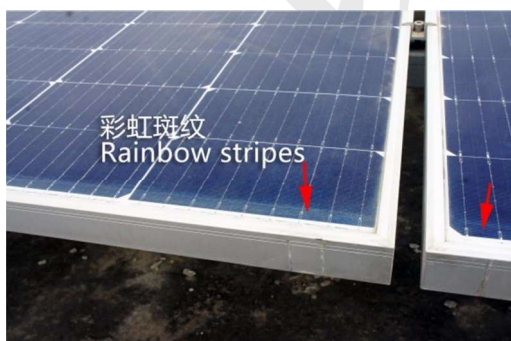
Figure 3 Moldy along the lower edge of the panels installed at an angle of 13 degrees
