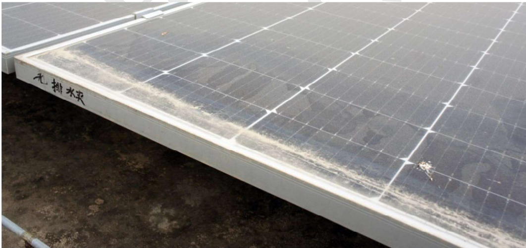
Figure 1. Soiling bands on the lower edge of the solar panels
